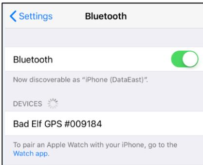
Select the external device and pair it with your mobile device. To do so, select *Pair* on your device and on Bad Elf receiver.
